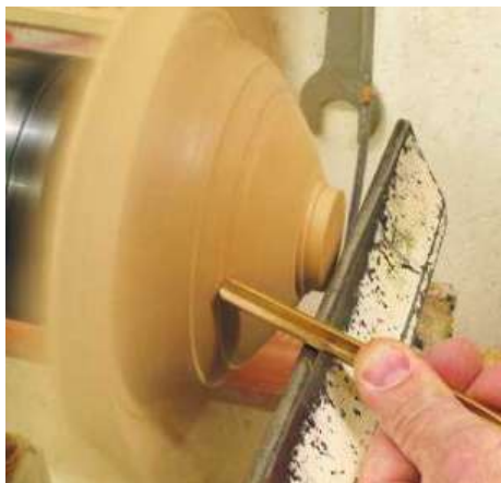
▲ Pic.16 It's difficult to get a good finish, so I decided to go back to using the 6mm bowl gouge with a light bevel rubbing cut, which will allow you to get a good sandable finish. Vibration did start to become a problem towards the end of the shape
